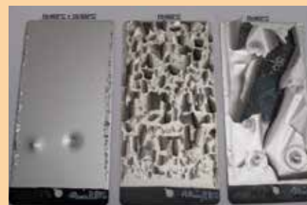
After curing at 280 °C 10 minutes: the phenylmethyl silicone SILRES® MPF 52 E (panel left) forms a stable film while silicone-acrylic (panel middle) and acrylic (panel right) are destroyed.
